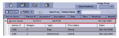
2. Select the correct processed images and manually transfer images to the desired Selected Network/PACS destination
